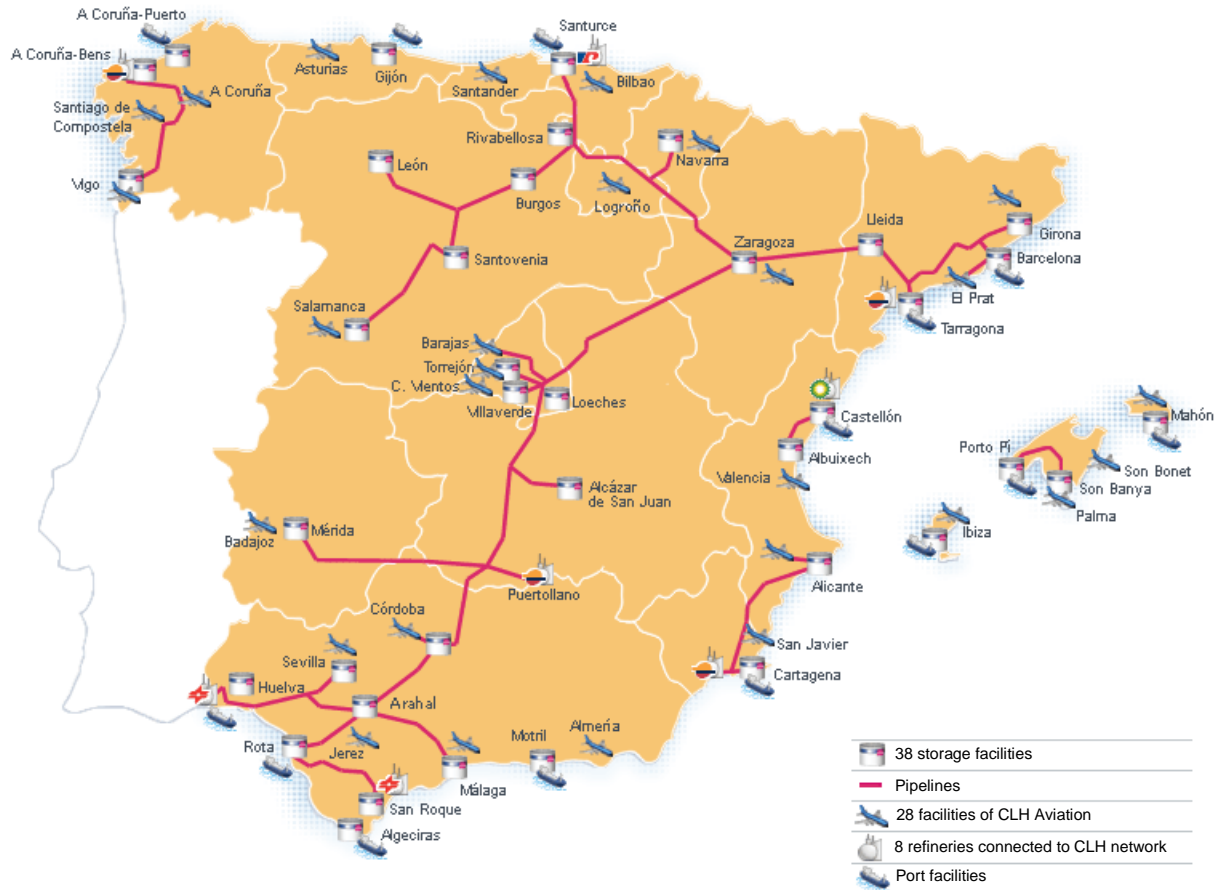
Figure 3. CLH pipeline network
