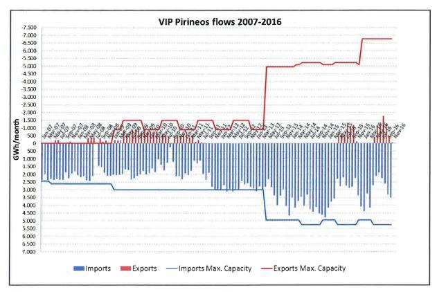
Figure 39. Interconnection capacity between Spain and France Source: CNMC and ENAGAS
